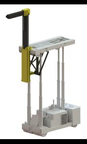
With the NEW Riggers Boom option, the TriLifter can reach an amazing 35' (10.6 m) with 25 tons!
