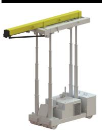
Increase the range of your TriLifter to 20' (6m) from the front of your unit. The pin-on jib extends with the power boom.
