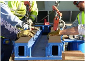
The HT500 features rigid steel tracks designed to carry loads over unsupported spans, is engineered to push loads up to 500 tons (454 tonnes), and has a working height of only 8" (205 mm).
