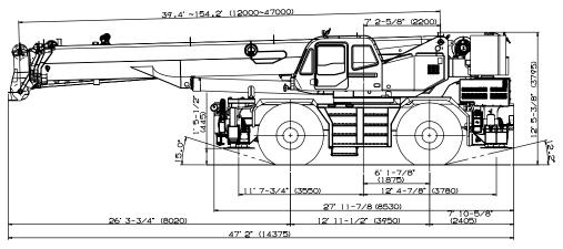
Note: Dimension is with boom angle at -1.5 degree.
