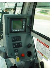
(LMI) is standard on all NBT45 machines. The LCD display is visible in full or low light and displays all crane load lifting values simultaneously. Includes Work Area Definition System (WADS).
