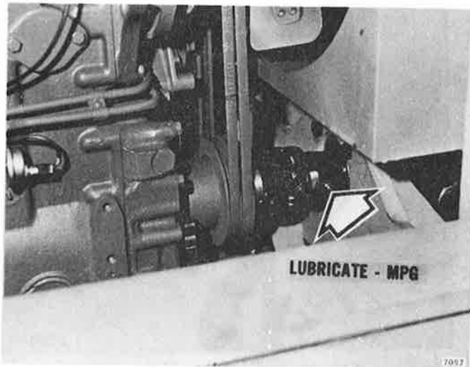
Figure 46 HYDRAULIC PUMP SLIP JOINT
