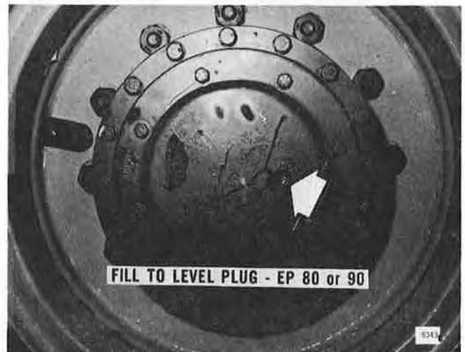
Figure 75 PLANETARY DRIVE LEVEL PLUG (ROCKWELL)
