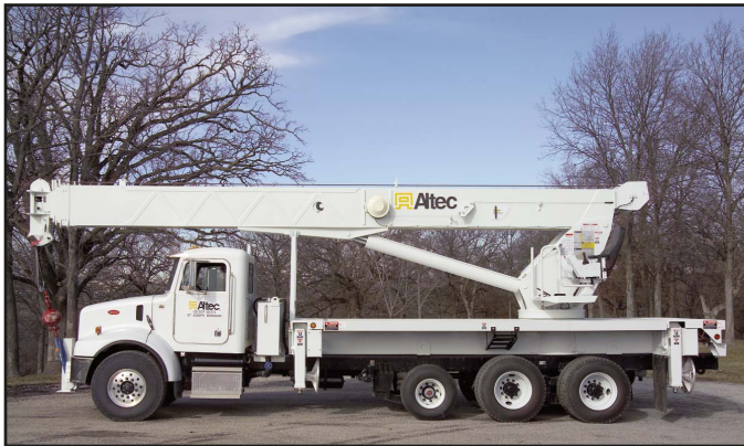
Vehicle Travel Height of 12.9 ft (3.9 m)
